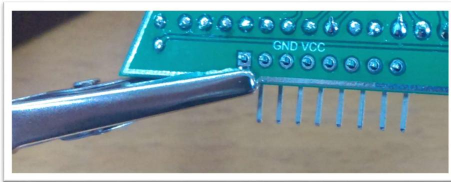
Here, we'll hold it from the left, and solder the right most connection, just to hold it in place. Make sure that the alligator clip is not bending the component or putting it in an awkward position; this too can take a bit of practise.
