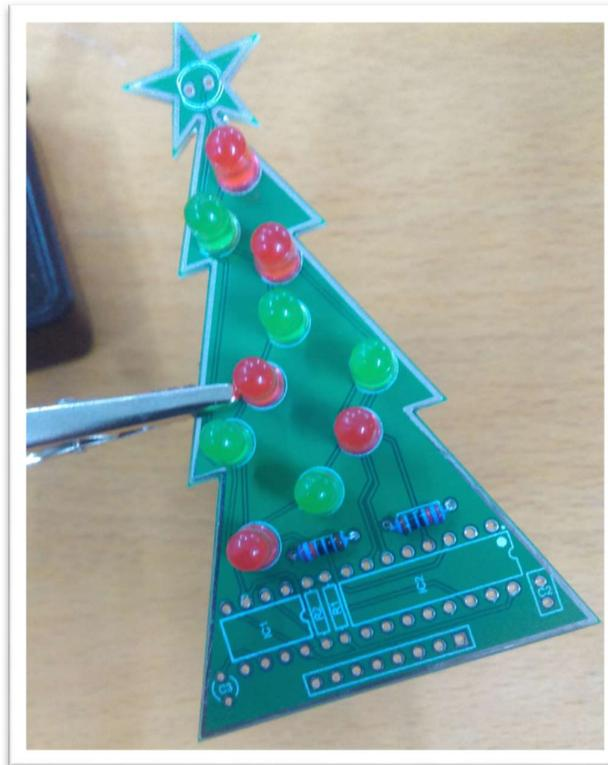
Similar to the LEDs: bend the legs so that they don't move, then snip them down to size. Heat from one side and apply solder from the other side, for each joint on the underside of the PCB.
