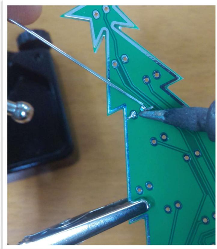
Here, you can see we have the PCB mounted in our “Third Hand” holder, TH1982. We apply the soldering iron to one side of the LED leg, touching both the leg and the pad underneath.
