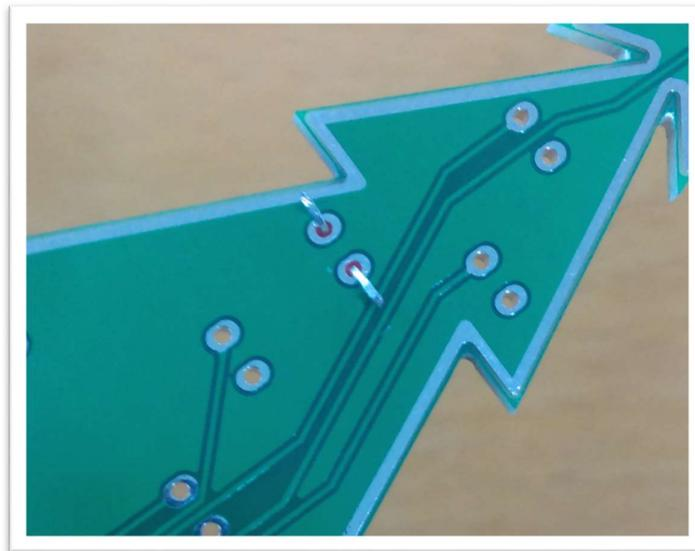
Once the legs are snipped, you can apply some solder to the joint. Read on in the next section for how.
