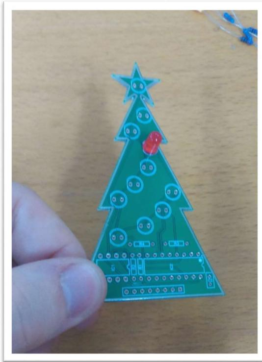
Then bend the legs of the LED so that the legs hold the LED into place and it can't drop out or wiggle around too much.
