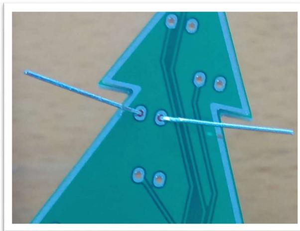
Once that is done, you will want to snip the legs of the LED much shorter. We do this so that the heat from the soldering iron is not wasted heating up the whole leg, only the small section close to where we want to solder
