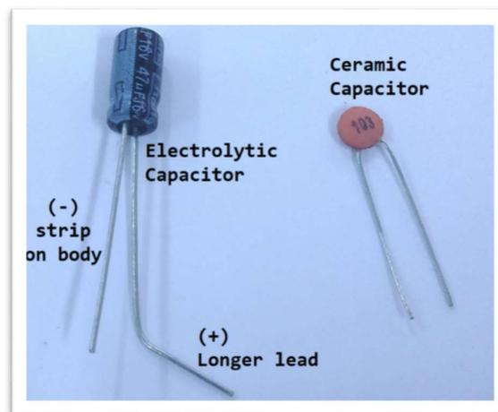
The ceramic goes into **C2** on the PCB board, which is next to the larger **IC2** socket. The electrolytic goes into **C3** which is next to the smaller **IC1**. If you asked "which way?" then congratulations, you're catching on. The supplied installation notes mention:
