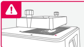
**NOTICE:** When installing the resin vat, please align the screws at the bottom of the resin vat with the platform grooves to avoid damage caused by the screws scratching the LCD panel.
