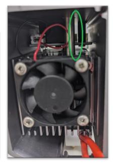
Next you will have to run the red wires up through the top of the circuit board and out the other side, similar to what was in the disassembly phase.
