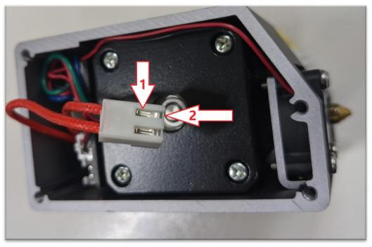
To unclip, gently press down on the small metal tab that is exposed in the connector, then pull the red wire to remove it from the housing. Do not push too hard as you can permantly bend the pin and make it difficult to clip back into the housing again.
