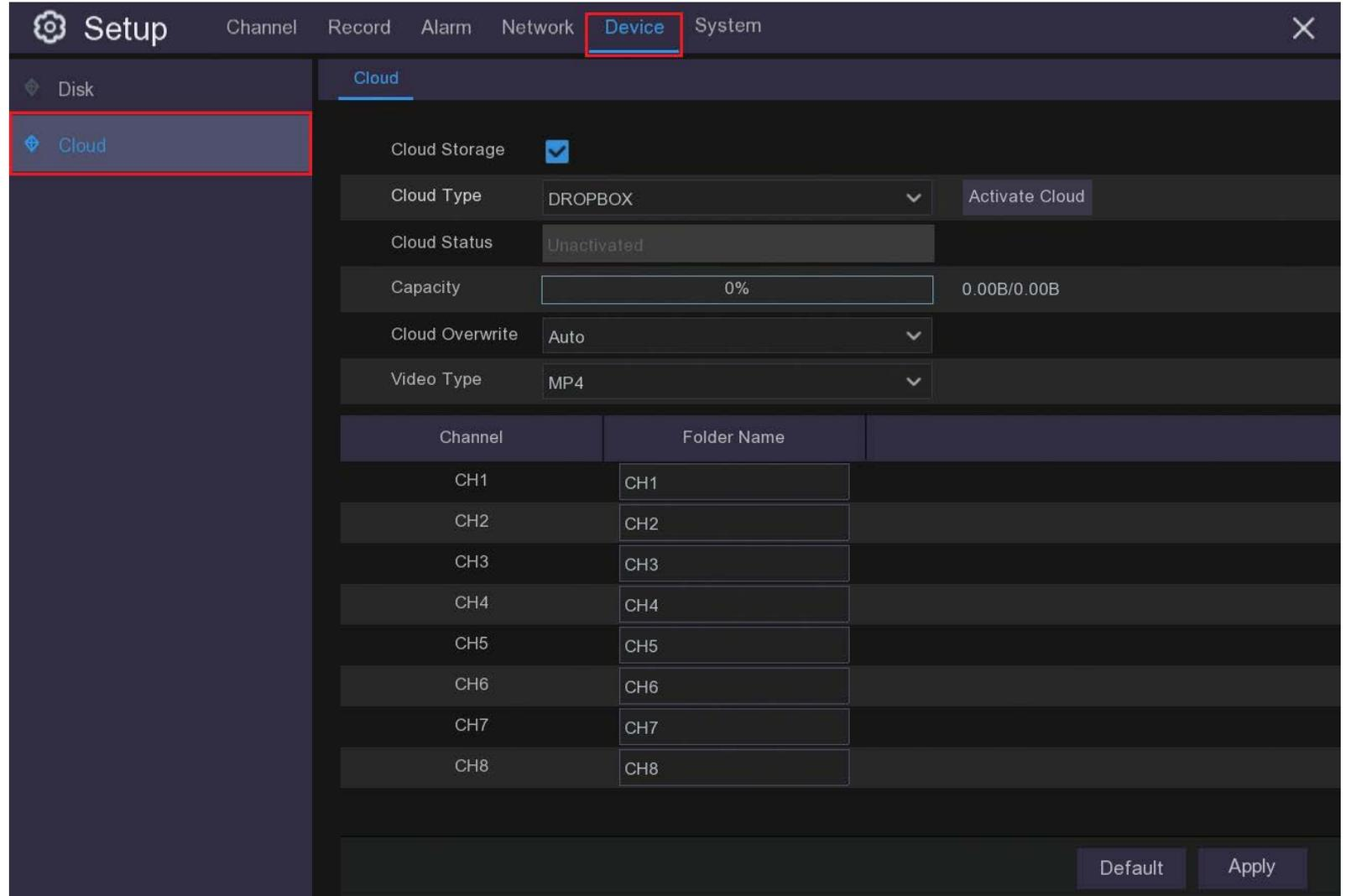
The screenshot shows the 'Setup' interface with the 'Device' tab selected. The 'Cloud' sub-tab is active, displaying various configuration options. The 'Cloud Storage' checkbox is checked. The 'Cloud Type' is set to 'DROPBOX'. The 'Cloud Status' is 'Unactivated'. The 'Capacity' is 0%, with a total of 0.00B/0.00B. The 'Cloud Overwrite' is set to 'Auto' and the 'Video Type' is 'MP4'. Below these settings is a table for configuring folder names for each channel.
