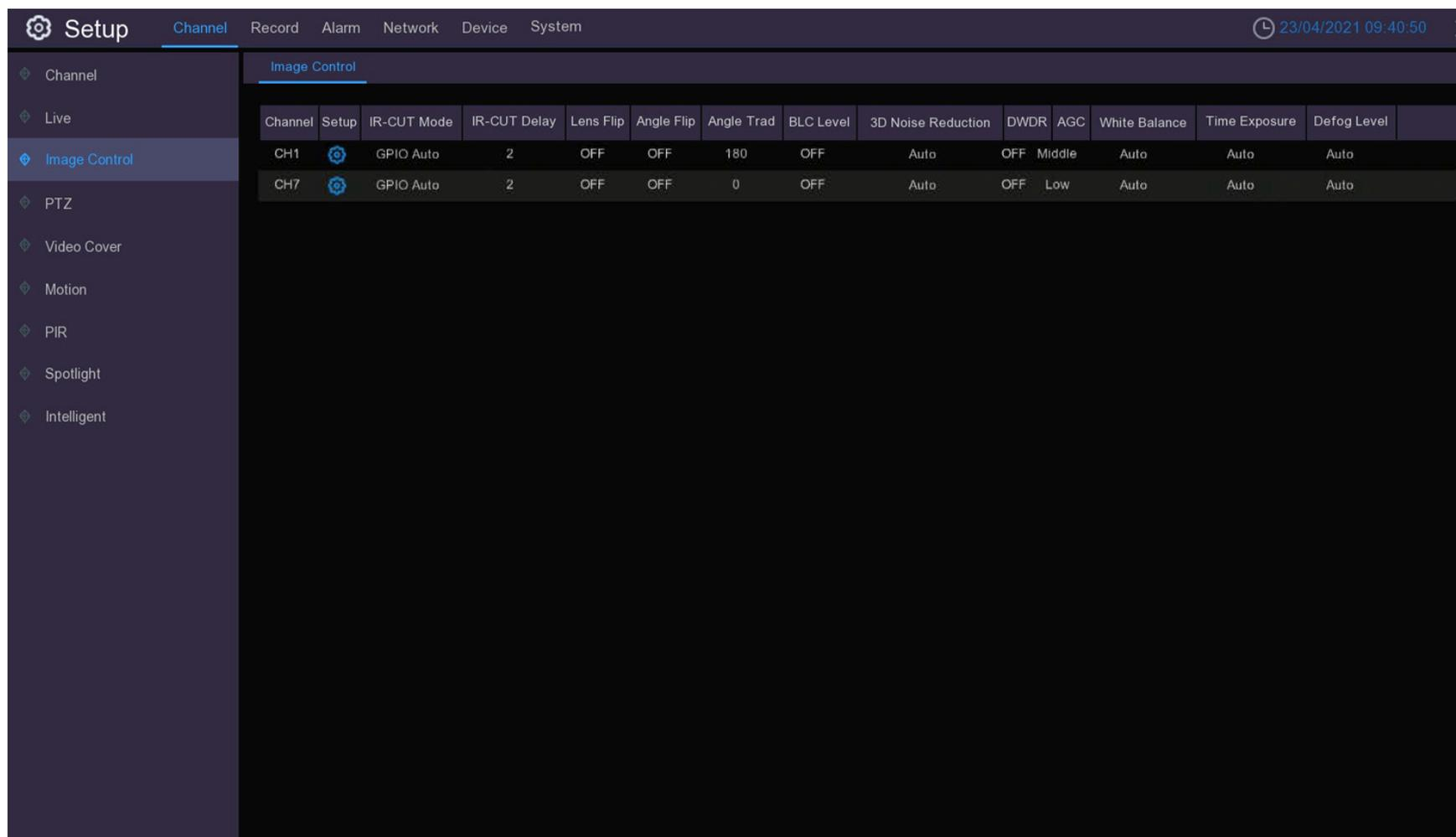
The screenshot displays the NVR setup interface. The top navigation bar includes 'Setup', 'Channel', 'Record', 'Alarm', 'Network', 'Device', and 'System'. The 'Setup' menu is expanded, showing options like Channel, Live, Image Control, PTZ, Video Cover, Motion, PIR, Spotlight, and Intelligent. The 'Image Control' menu is selected, showing a table of settings for two channels: CH1 and CH7.
