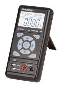
0.3 to 30V, 0 to 3.75A Portable Laboratory Power Supply
