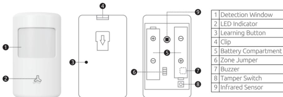
**Infrared Sensor:** Detects the infrared rays released by human body motion.
