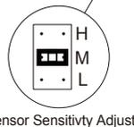
Sensor Sensivity Adjust
