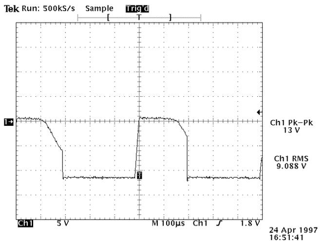
**Fig.6:** this scope waveform shows the effect when both diode D2 and the 0.22µF capacitor are fitted to the circuit. Note that the capacitor has a filtering effect which acts to remove most of the hash generated by the motor's commutator.
