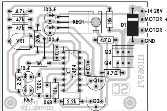
Fig.7: the component overlay for the PC board.
