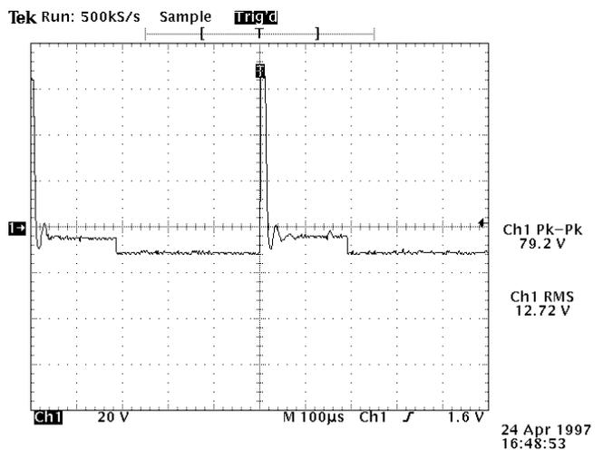
**Fig.4:** this waveform shows the circuit set for the same output as for Fig.3 but driving a motor instead of a resistive load. The scope's vertical sensitivity has been changed to 20V/div instead of 5V/div. Notice the enormous spike voltage (amounting to almost 80V p-p) each time the Mosfets turn off. This spike voltage is enough to blow the Mosfets because their Drain-Source voltage rating ( $V_{DS}$ ) is only 60V.
