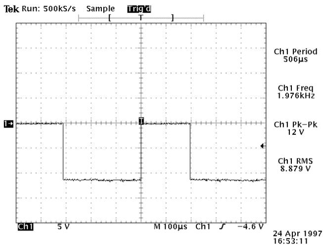
**Fig.3:** this scope capture shows the waveform across a resistive load which could be a heater element or an incandescent lamp. Notice that the waveform is a clean pulse with a duty cycle of about 74%. This gives a voltage of about 8.8V across the load.
