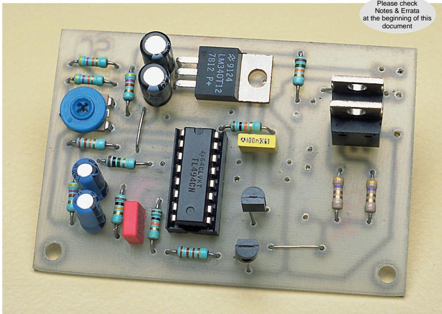
**This small PC board will provide speed control of 12V or 24V motors drawing up to 20A. Not shown on this prototype board is the input protection diode D1**
