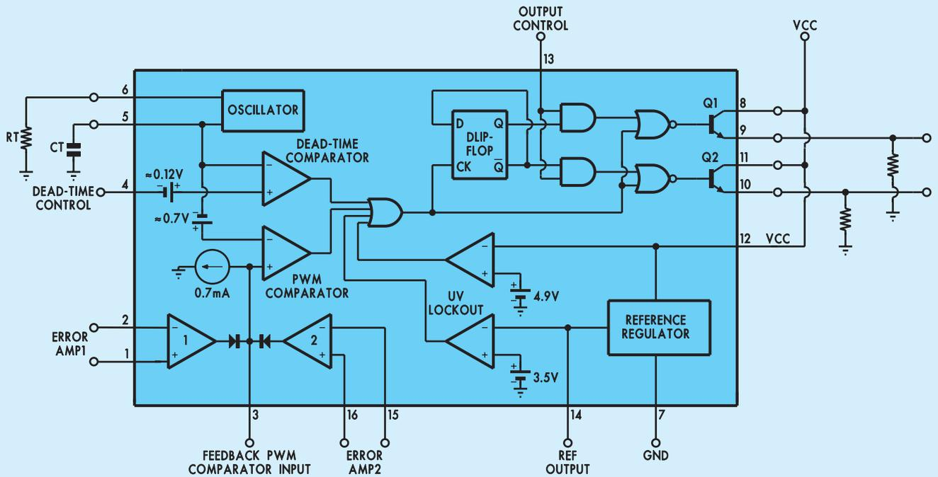
**Fig.2: functional block diagram of the TL494. This chip is intended mainly for switchmode power supplies but we have adapted it to control motors and resistive loads.**
