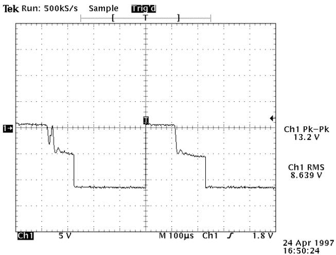
**Fig.5:** this waveform was produced with the same circuit conditions as for Fig.4 but with D2 connected across the motor to clip the voltage spikes. We now see the motor's back-EMF during the Mosfet "off" period, showing a value about half of that applied by the control circuit.
