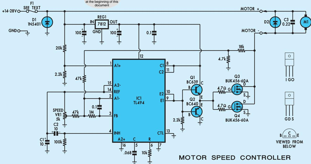
Fig.1: the heart of the circuit is a TL494 pulse width modulation (PWM) controller. It varies the output voltage fed to the motor by rapidly turning Mosfets Q3 & Q4 on and off. Note that diode D2 is essential to the circuit operation.
