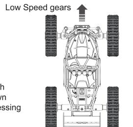
When the car is in high speed, it will slow down on rough roads by pressing low speed.
