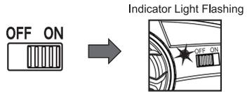
First, turn on the power supply of the car and transmitter. The transmitter automatically searches for the frequency and the indicator light flashes. When the transmitter indicator light Extinguish, means match successful. All functions of the transmitter can be used normally. If the car does not respond, turn off the car and transmitter Power and re-operate the frequency again.
