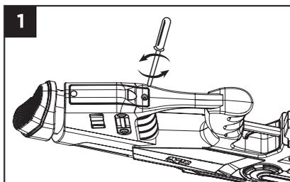
1 Use a screwdriver to remove the battery cover.
