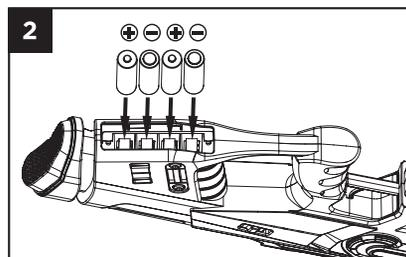
2 Insert 4 x AA batteries. Make sure the batteries are inserted with the correct polarity.
