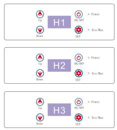
H3 should be set when the product is connected to car power, and H2 or H1 should be set when it is connected to a portablebattery or other back-up batter. Because of the different outputvoltages between vehicles, the battery gear can be set from H3 to H2 from H2 to H1 if there is a voltage protection code F1shown on the panel. The battery gear should be set to H if thoroduct will keep working after turning off the car engine, or the product may drain the battery.
