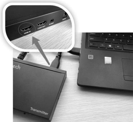
**03** Connect the Transmitter to your media output device through the "HDMI IN" port.
