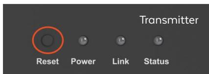
**07** When the display screen shows "SearchingTX", short press the "Reset" button in turn on the Receiver and the Transmitter.
