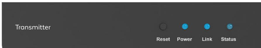
Power LED is solid, Status LED flash frequency is faster than Link LED
