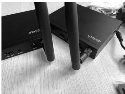
**01** Install antennas for Transmitter & Receiver.
