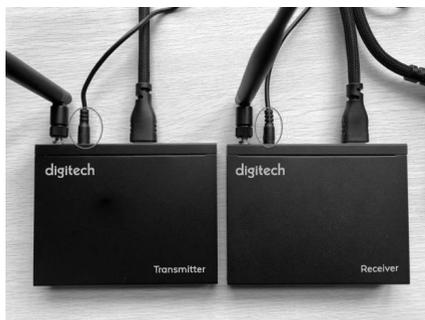
**04** Connect power to Transmitter and Receiver separately.
