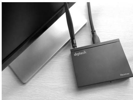
**02** Connect the Receiver to your output display through the "HDMI OUT" port.
