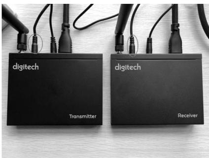
**03** Connect the Receiver and Transmitter with the 3.5mm male to male cable.
